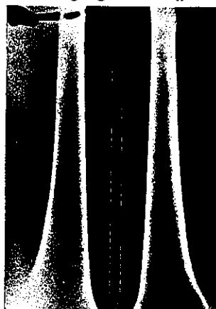
FIG. 6 - SCHLIERENPHOTOGRAPH OF THE FIELD OF TEMPERATURE IN FRONT OF A PLANE VERTICAL PLATE 12 cm HIGH AT A TEMPERATURE OF ABOUT 70 C ABOVE THAT OF THE SURROUNDING. THE DOTTED LINE IS THE CONTOUR OF THE SHADOW OF THE PLATE IF NOT HEATED.
